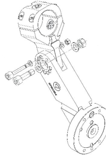
Kemppi Robot Gun Mount T4 is a solid bracket without collision sensibility. It is recommended that the robot itself is equipped with the collision sensing ability, when Kemppi Robot Gun Mount T4 is used. Gun orientation can be adjusted in 30 degree steps.
