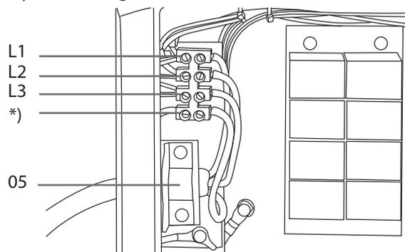
\*) In cables of S type there is a protective grounding conductor coloured green-yellow.
