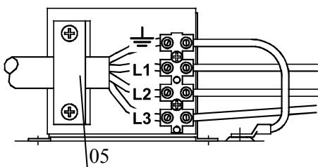
The cable is entered into the machine through the inlet ring on the rear wall of the machine and locked with a cable clamp (05). The phase conductors of the cable are coupled to connectors L1, L2 and L3. The earth protection coloured green-yellow is coupled to connector marked with earth protection symbol (⏚). If you are using 5-conductor cable, you must cut the zero conductor to the level of the cable's protective shield.
