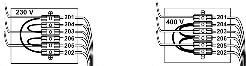
By delivery from the factory the machine has been connected for mains voltage 3~ 400 V. In order to change the mains voltage, remove the side plate of the machine. Change the connections according to the enclosed diagram. You find the corresponding wiring diagram on the instruction label, which is under terminal block.
