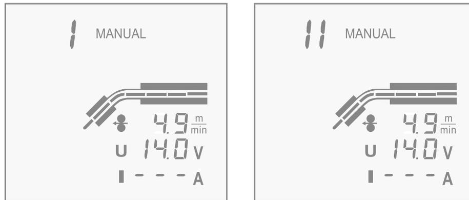
In Manual mode you can select from two different arc dynamics settings. Press Manual mode button (Arc Dynamics control on MinarcMig 170 model) once to pre-select either arc dynamic value I or value II. Changing between setting I and setting II will adjust the short circuit characteristics to suit different welding applications.
