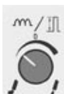
When you adjust welding dynamics, the adjustment value -9...0...9 is shown in display V, which otherwise shows set value / welding voltage. Value of dynamics is shown in display for approx. 3 s after adjustment.
