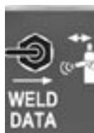
Use of WELD DATA switch retrieves welding parameters, wire feed speed, welding current, welding voltage which were used when welding was stopped last. Welding values are indicated in display for so long you are using the WELD DATA switch, and are stored until you press again the start switch for gun.
