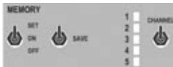
SELECTO is the name for the operation which allows you to store welding parameters. You can save five sets of MIG welding values. Parameters which can be stored are wire feed speed, welding voltage and welding dynamics.
