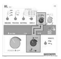
If interconnecting cables between wire feed unit and power source are not used, set cable compensation at position zero.
