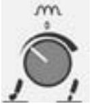
MIG and MMA welding dynamics are adjusted with the same potentiometer. When you adjust welding dynamics the adjustment value -9...0...9 is shown in display V, which otherwise shows set value/welding voltage. Value of dynamics is shown in display still for approx. 3 s after stopping the adjustments.
