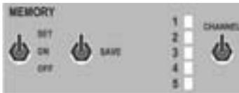
SELECTO is the name for the operation in which you can store welding parameters for memory channels for reutilization. You can store to memory five sets of MIG/MAG welding values. Parameters which can be stored are wire feed speed, welding voltage and welding dynamics. Stored values are kept in memory though power is switched off from unit.
