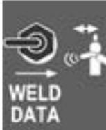
Use of WELD DATA switch retrieves to displays welding parameters, wire feed speed, welding current, welding voltage which were used when welding was stopped last. Welding values are indicated in display for so long as you are using the WELD DATA switch and are kept in memory until you press again the start switch for gun.
